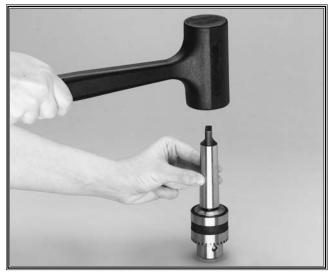
Figure 19. Seating the arbor into chuck.
